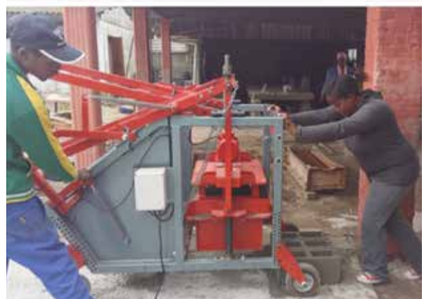
Trainees in the TWU garden pot centre learn the skills and trade of brick and block making.
