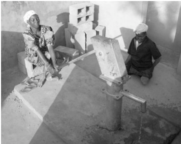
Figure 4.15 Disabled women from the local community assist in preliminary tests of end-seat positioning and height.
