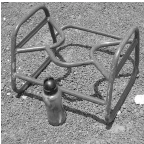
Figure 6.23 Equipped with bracing below the seat level, this chair is designed for cleaning from the rear (note the curved brace in the rear), but can also be turned around and used by those wishing to clean from the front.
