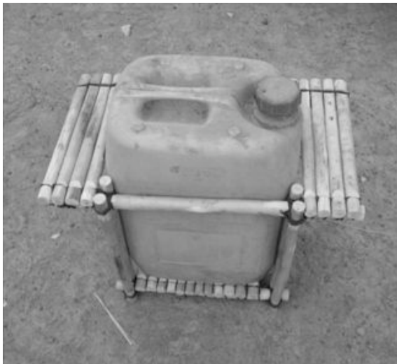
Figure 5.15 A wooden prototype of jerry can holder (“porte-bidon”). These are considerably less costly than metal holders but are not as robust. This prototype is equipped with side handles almost twice the necessary width.
