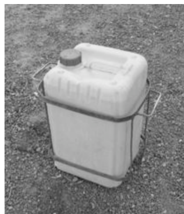
Figure 5.14 One of the final prototypes of jerry can holders (“porte-bidon”) developed during the Study. Note the minimal amount of metal used and the handles placed on the narrower sides of the container for greater ease of lifting on and off the head.
