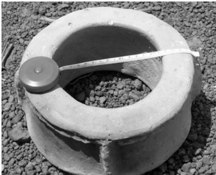
Figure 6.14 Terra cotta (baked earth) latrine seat for traditional latrines; fabricated by a local potter.
