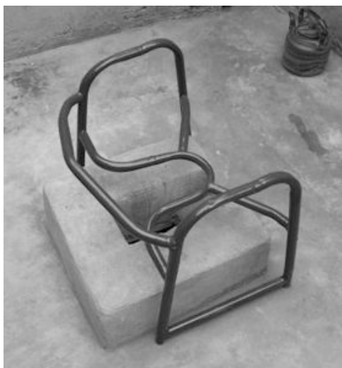
Figure 6.24 Low placed support bracing on the side of this latrine seat makes it more stable and less likely to sink in the ground if used on an earthen surface (such as is found in most traditional latrines).
