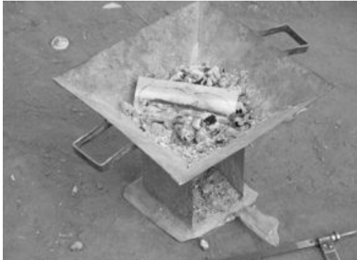
Figure 5.16 Heating the thin flat strip of metal (e.g. aluminum) which will be placed briefly between the container and the handle to be attached. This step will heat both sides for welding.
