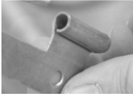
Figure 5.40 The sheath portion of a discarded metal hinge can be removed, inserted into the wooden support frame of a tipper, and serve as a protective sheath for the pivot bolt; thus reducing wear and tear on wooden parts.
