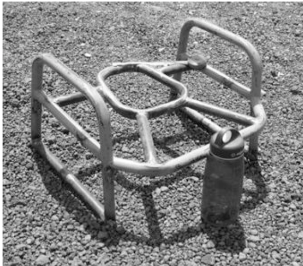
Figure 6.17 An early metal latrine chair prototype developed during the Study. While functional and sturdy, this design with an enclosed seat and adjacent bracing limits hand access for cleaning (either from the front or from the rear).
