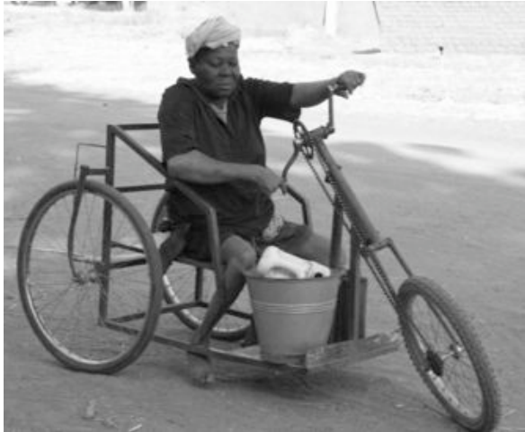
Figure 5.23 A disabled woman uses the foot platform of her tricycle to transport water, as the low center of gravity enhances container stability and reduces splashing, but the placement of the container leaves little room for her legs. Notice how the support frame intersects the center of the foot platform, limiting space for carrying objects.
