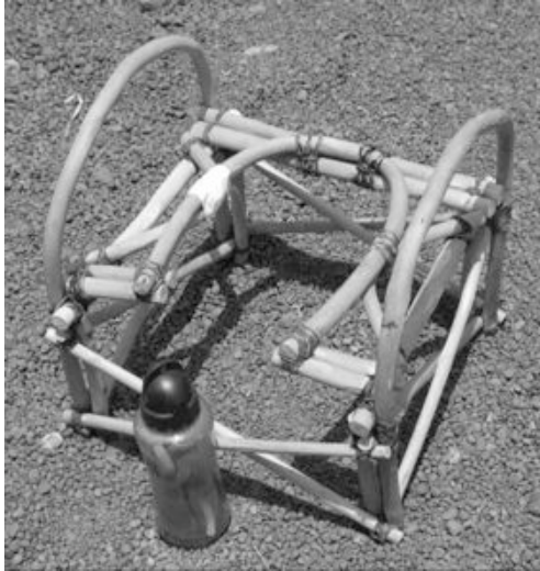
Figure 6.27 Chaise Bagayogo: The standard-sized wooden latrine seat developed by the Study which can be used from either direction, depending on preference for front or rear cleaning. The chair is light, sturdy, locally fabricated and low-cost.
