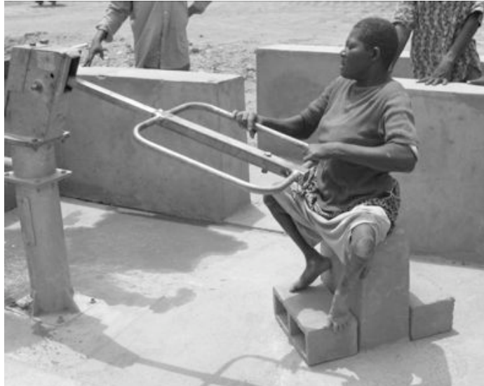
Figure 4.20 A disabled woman, with lower-body disability and limited use of one arm, assists in testing the positioning of a side-seat with a rectangular-handle attachment.
