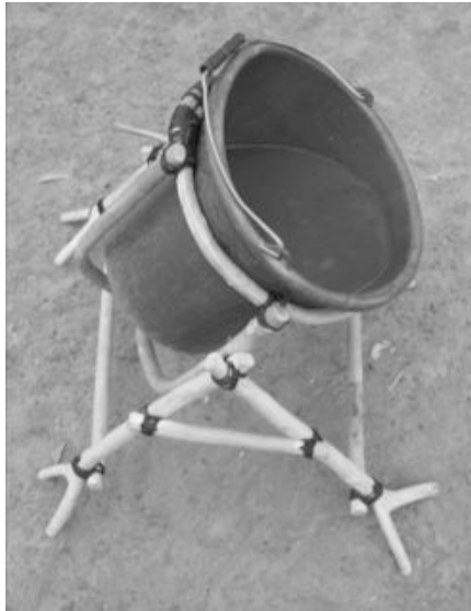
Figure 5.37 An early prototype of the wooden bucket tipper, made by local artisans in the Tominian region of Mali.
