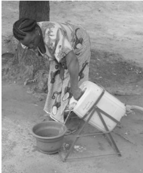
Figure 5.30 A disabled woman tests an early jerry can tipper prototype. Note the overly wide base of the support frame, which impedes good placement of the receiving container directly under the jerry can outlet. The tipper also lacks a handle at the base of the holder, requiring awkward handling from the top of the jerry can.
