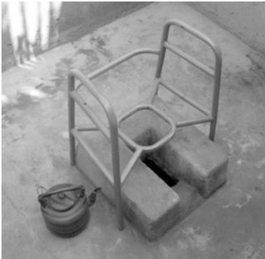
Figure 6.19 This early latrine chair prototype was developed for use by a disabled person needing assistance to walk from her room to the household latrine and to squat while using the latrine. The handles are made at a height which can easily be grasped from an upright, walking position. The handles and other side bracing provide support for lowering and raising herself from the latrine.
