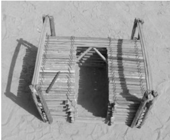
Figure 7.2 Raw material and local craftsmanship may vary from region to region in West Africa. Local artisans in the Zinder area of Niger developed this initial latrine seat prototype using dried palm branches and wire.
