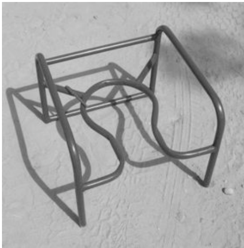
Figure 6.22 This metal latrine chair is fabricated with a standard seat for front cleaning. This seat functions well on hard surfaces, but the stand-alone front legs may sink into the ground if used on an earthen surface.
