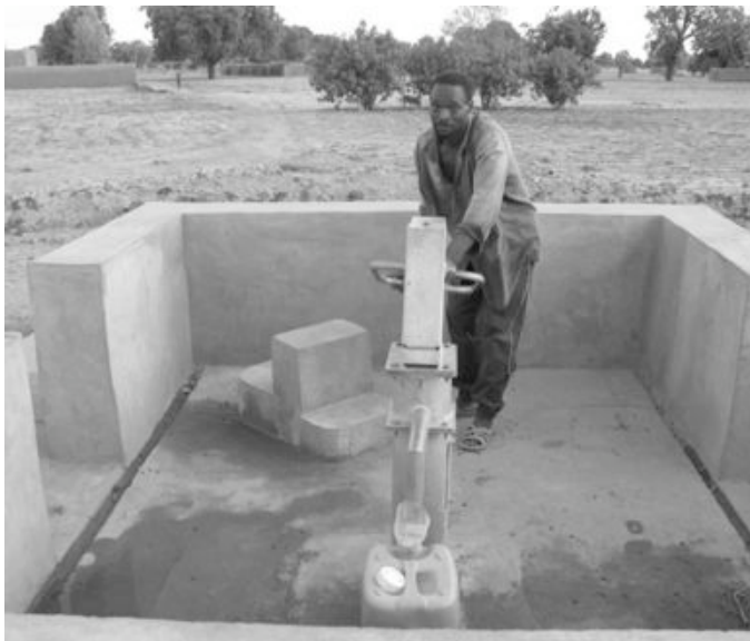
Figure 4.22 An able-bodied man demonstrates use of the pump equipped with the completed side-seat and rectangle-handle attachment. The side-seat is positioned at about 45° from the pump handle, with a high approach step in the rear and a lower leg/foot stabilizer in the front.
