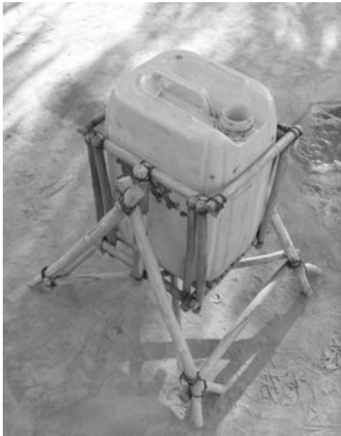
Figure 5.39 A final prototype of the wooden jerry can tipper.
