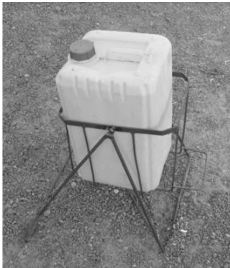
Figure 5.35 Final version of a jerry can tipper.
