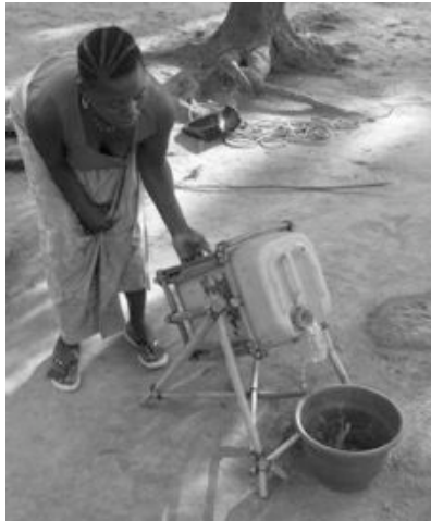
Figure 5.43 Woman with limited upper-body mobility uses a wooden jerry can tipper in the home.
