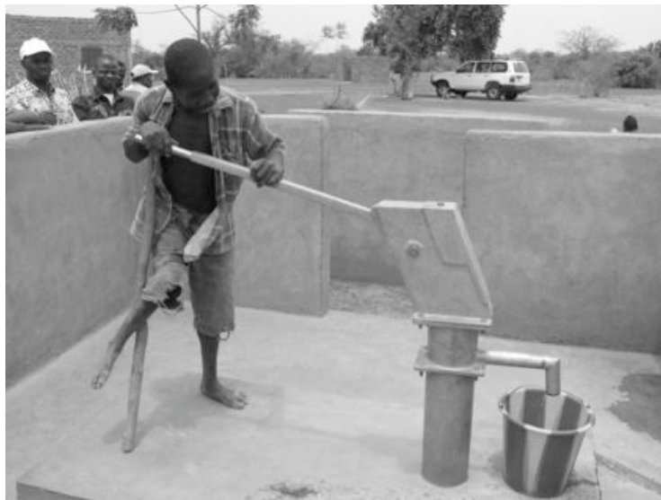
Figure 2.15 A young disabled man trying to simultaneously pump and hold himself upright with his cane. In this position, he is unable to produce a steady flow from the pump.
