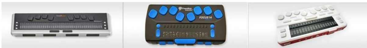
Figure 6. Exemples de tablette Braille (Brailiant 40 (Humanware), Focus 14 (Freedom Scientific) et Braille Sense U2 Mini (Hims)).
